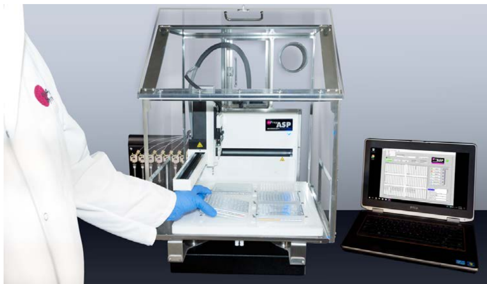
Figure 1: ASP-1000 setup with mPrep/s capsules and reagent plates.
