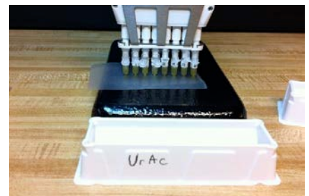
Figure G: Placing capsules on Parafilm during staining.
