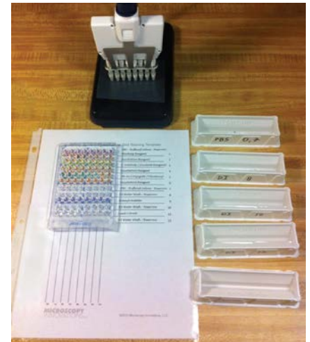
Figure A: Preparation of equipment and supplies. Use a lab stand and clamp to hold the pipettor upright, the protocol template, and reservoir troughs.
