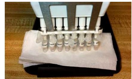
Figure I: Blotting excess fluid from mPrep/g capsules.
