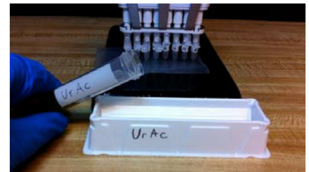
Figure F: Pouring a reagent (in this case uranyl acetate stain) into a reservoir.
