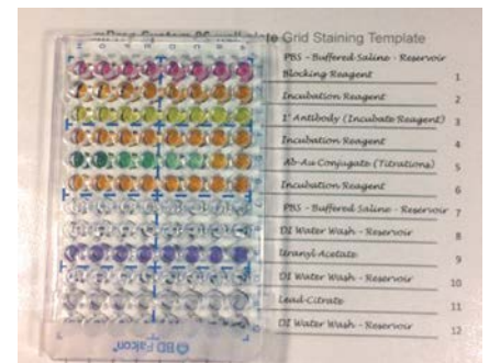
Figure B: Microplate containing reagents placed on protocol template in portrait orientation to use with 8-channel pipettor.
