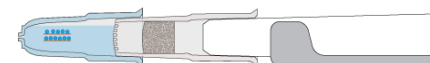
Figure 3: Enhancing nanoparticle sedimentation. Setting mPrep/g capsules horizontally can enhance sedimentation of nanoparticles onto filmed grids.
