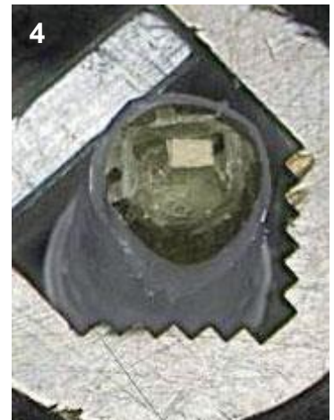
Figure 4: mPrep/s capsule with epoxy block directly clamped in microtome chuck, trimmed through capsule and faced for sectioning.
